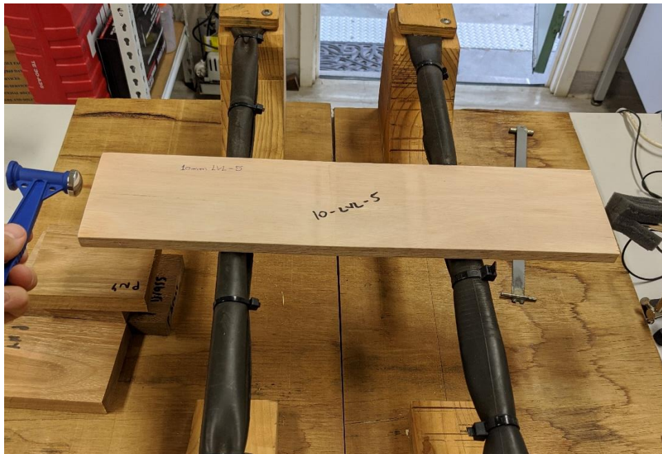
Figure 1: Acoustic assessment of LVL sample.
