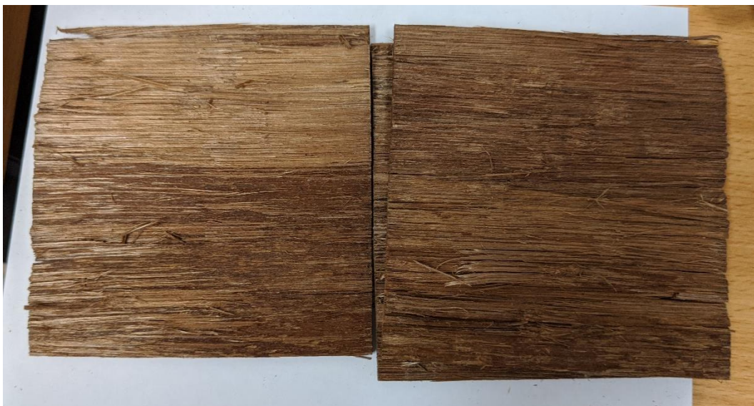
Figure 9: 16-12-LVB-7 Bond Quality test specimen showing an area of poor adhesion.
